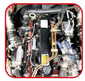
Cummins D4.0EVID160 TURBO DIESEL INTERCOOLER
